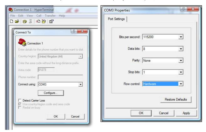
On the terminal screen, type "AT" to check the "OK" response from the modem
