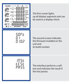
\*After a short delay, the screen will display active energy measurements.
