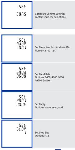
On completion of the entry procedure, press the PhS button and you will return to a parameter screen
