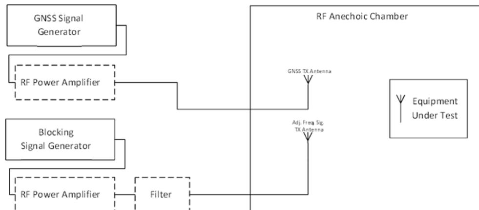
**Figure 5-2: Radiated measurement setup for EUT receiver blocking**
