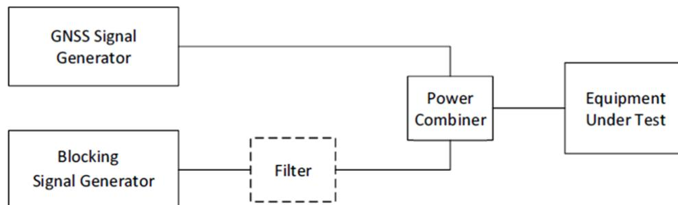
Figure 5-1: Conducted measurement setup for EUT receiver blocking
